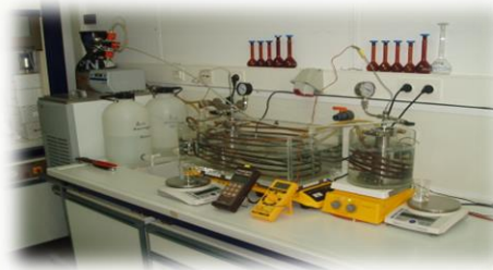
Membrane concentration of high-added value compounds contained in effluents - Schematic diagram and a view of lab-unit.
