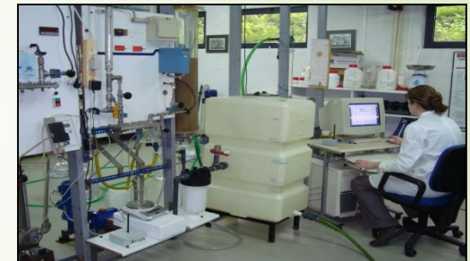
Pilot unit for continuous monitoring of scaling potential in desalination plants.
