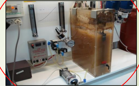
Membrane bio-reactor (MBR) pilot unit
