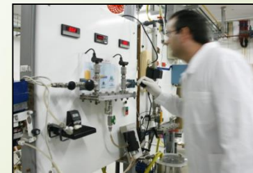
Special equipment for characterization of desalination membrane performance
