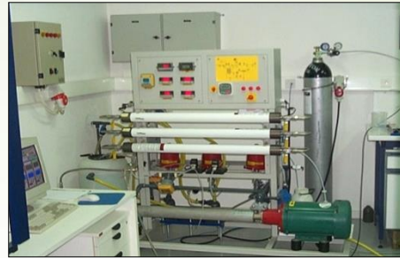
Medium pressure membrane pilot unit (LPRO / NF)
