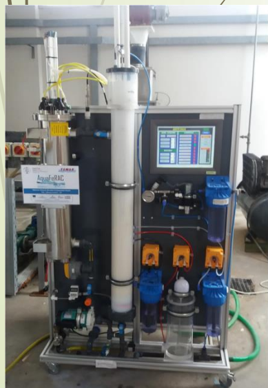
PMR Pilot Plant - Mineralization of toxic micro-pollutants
