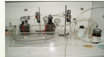
Membrane extraction unit for olive polyphenols recovery - Schematic diagram and a view.
