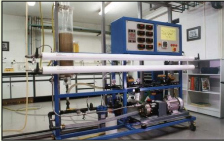
High pressure membrane pilot unit (RO)
