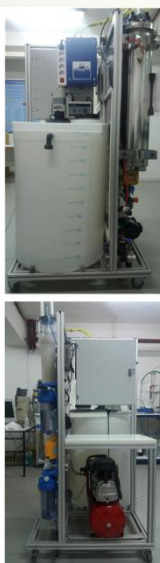
PMR Pilot Plant - Mineralization of toxic micro-pollutants
