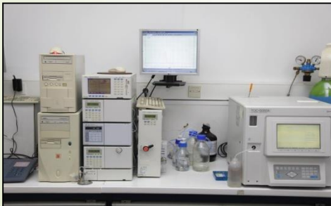
GC/MS, GPC/HPLC, GC, TOC, Ion Chromatograph Systems, Particle Size and \zeta -potential measurement equipment, Spectro-photometers; equipment for BOD 5 , COD, SDI
