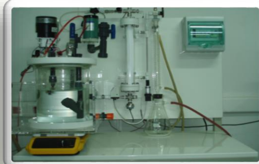
Agricultural wastes fermentation, coupled with membrane distillation for continuous bio-ethanol recovery Schematic representation and a view of laboratory pilot unit.
