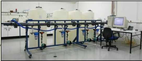
High pressure membrane pilot unit (RO)
