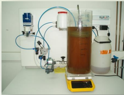
Schematic diagram and a view of lab-scale pilot unit for pre-treatment (clarification by UF membranes) of agro-industrial wastewaters containing high-added value substances
